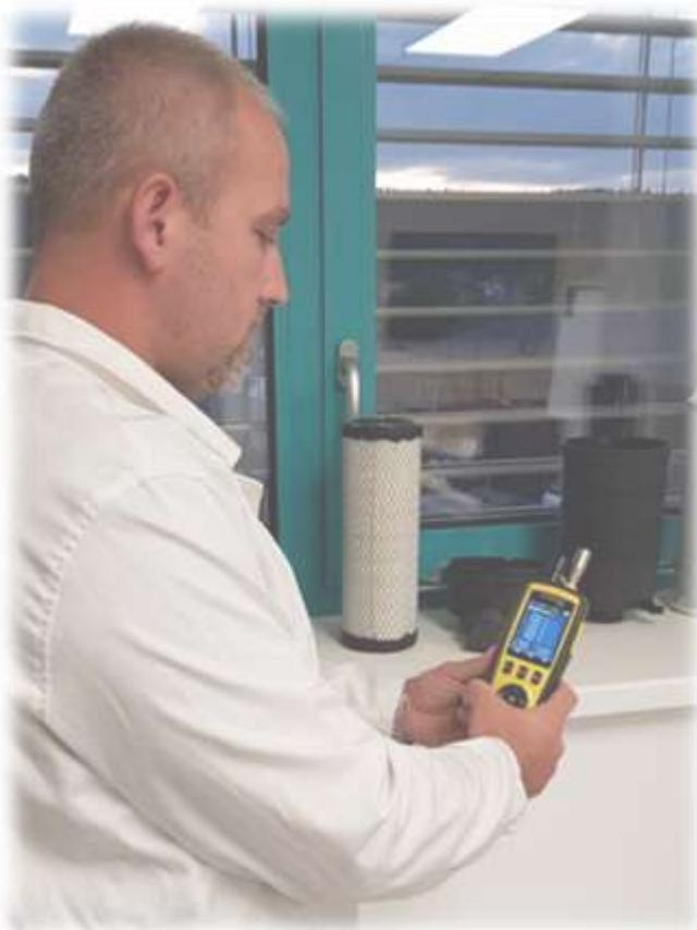
**Performance measurement of particle / contamination concentration** in accordance with standard ISO-21501-4
